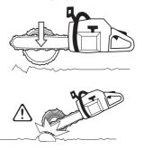
If it is possible (can you turn the log?) stop cutting about 2/3 of the way through the log.
